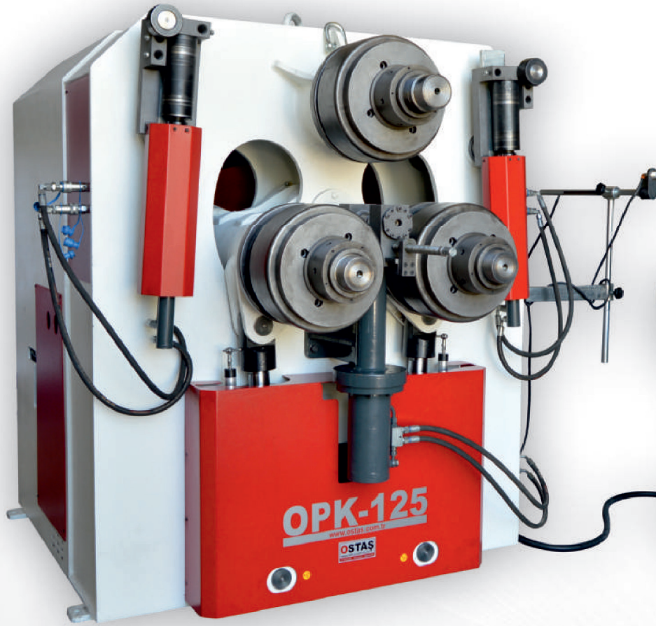
Hidrolik motor ve planet redüktör ile tahrikli valsler All (3) three rolls are driven with hydraulic motor and planetary gear box
