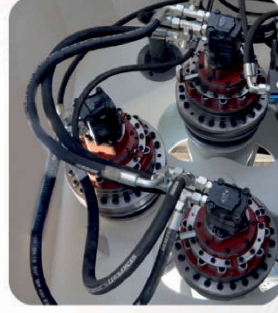
Hidrolik motor ve planet redüktör ile tahrik valesler All (3) three rolls are driven with hydraulic motor and planetary gear box
